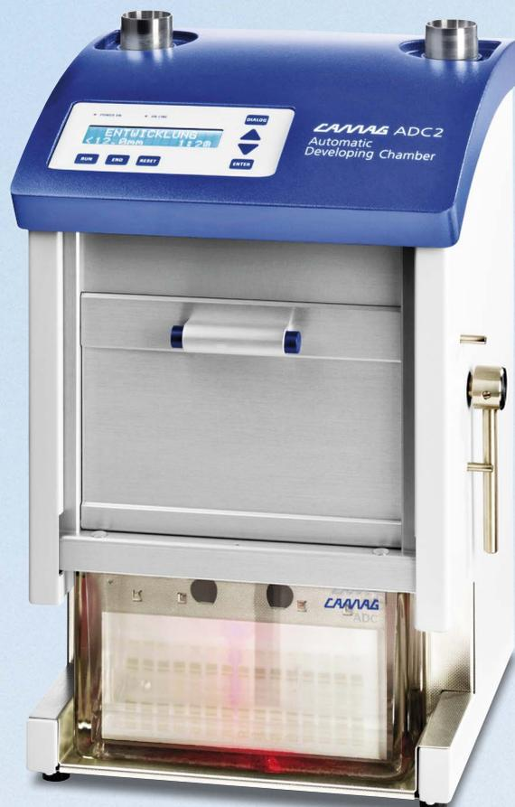
The Automatic Developing Chamber offers convenience, safety and reproducibility for the isocratic development of TLC/HPTLC plates and foils with the format 20 × 10 and 10 × 10 cm.
