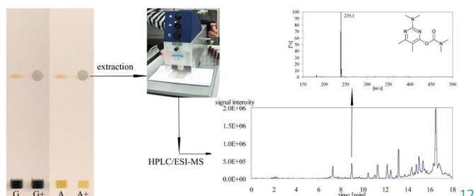
Extraction of a target zone with the TLC-MS Interface followed by LC-MS, total ion current chromatogram (TIC) of an apple extract spiked with a mixture of pesticides of various substance classes (A+) and mass spectrum of the peak with Rt=9 min (pirimicarb, m/z 239.1, [M+H]<sup>+</sup>).
