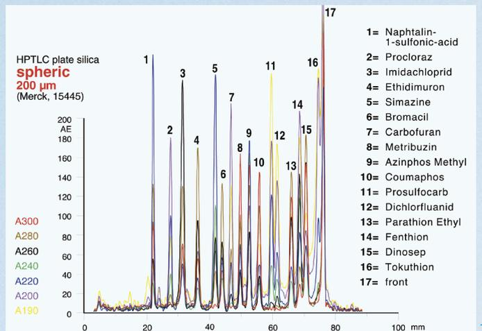
Densitogram (MWL scan) of an AMD chromatogram of pesticides HPTLC plate Lichrosphere silica gel 60 F<sub>254</sub> Merck
