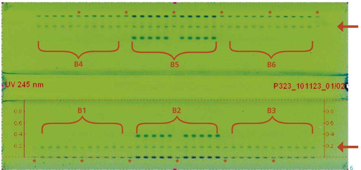
60 samples (6 batches, B1–B6) and 12 standards\* were applied onto one HPTLC plate; Coenzyme Q10 is seen at  $R_f \approx 0.20$ . In the Q10-batches on the center tracks vitamin B2 and vitamin E are also present ( $R_f \approx 0$  and  $0.4$ ); (\*NOTE: For better visualization in this figure the application volume was increased to  $6 \mu\text{L}$ ).
