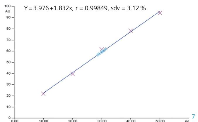
Calibration function for Coenzyme Q10 at UV  $282 \text{ nm}$ . Measurement of 10 samples and 5 standards using linear calibration (P323\_101011\_03).
