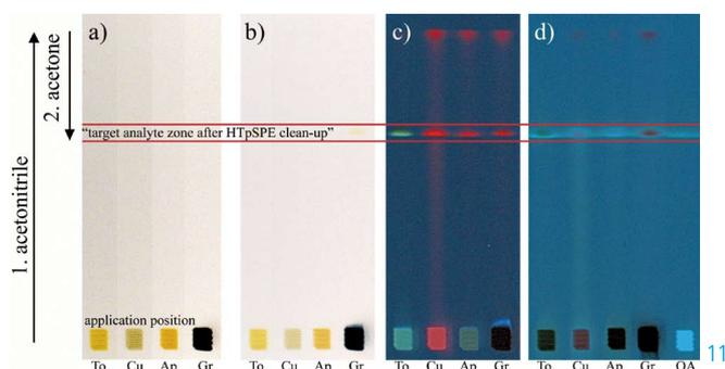
Separation of matrix and pesticides on TLC aluminum foils silica gel 60 NH<sub>2</sub> F<sub>254s</sub> (tomatoes (To), cucumbers (Cu), apples (Ap) and red grapes (Gr); oleic acid (OA) was applied as a fatty acid example); before development under white light (a), after development under white light (b), UV 366 nm (c) and UV 366 nm after derivatization with primuline (d) (reprinted from [1] with permission).
