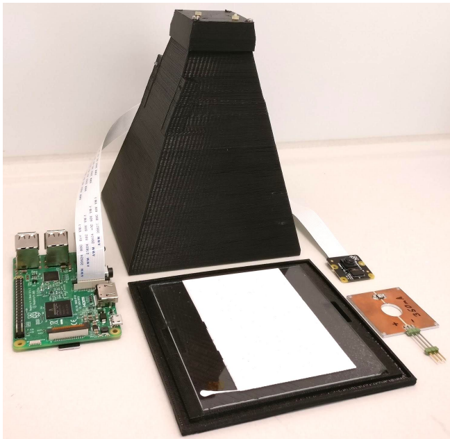
Visualization chamber with raspberry pi, camera and UV-LED
