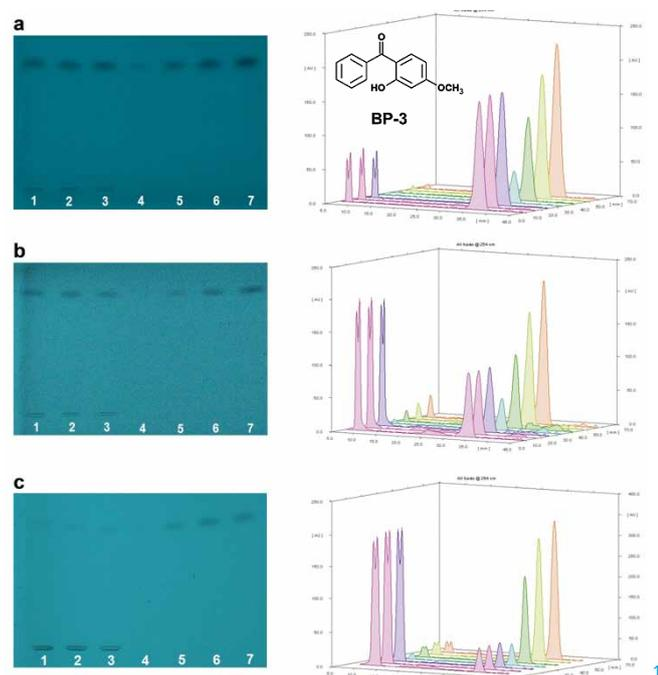
Chromatograms and densitograms of amino plates with BP-3 after storage in the dark at room temperature (a), heating at 33 °C (b), and UV irradiation irradiated at 350 W/m<sup>2</sup> (c), 1 h each (with permission from [1])
