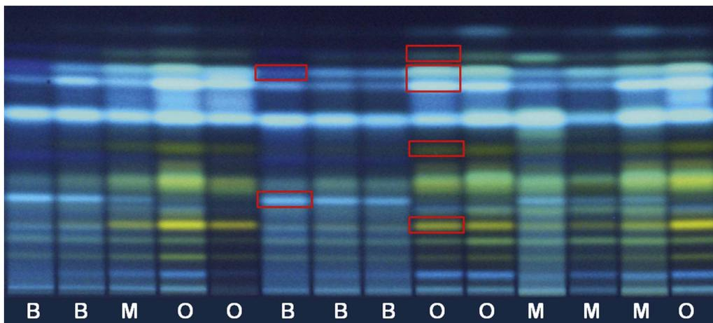
HPTLC chromatogram of German propolis samples of orange (O), blue (B) and mixed (M) types with characteristic markers (marked red)
