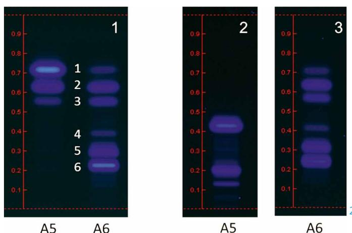
HPTLC separation of fractions and detection under UV 366 nm with
