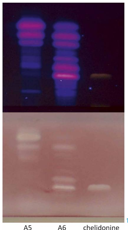
TLC separation of the 2 fractions of Galbanum as well as chelidonium standard with chloroform – ethyl acetate – methanol 50:5:1 under UV 366 nm (top) and with AChE inhibition (down)
