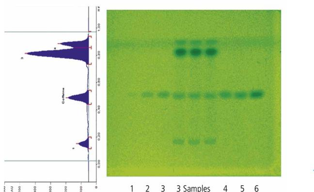
Absorbance measurement (254 nm) of the middle shampoo sample in the chromatogram under UV 254 nm
