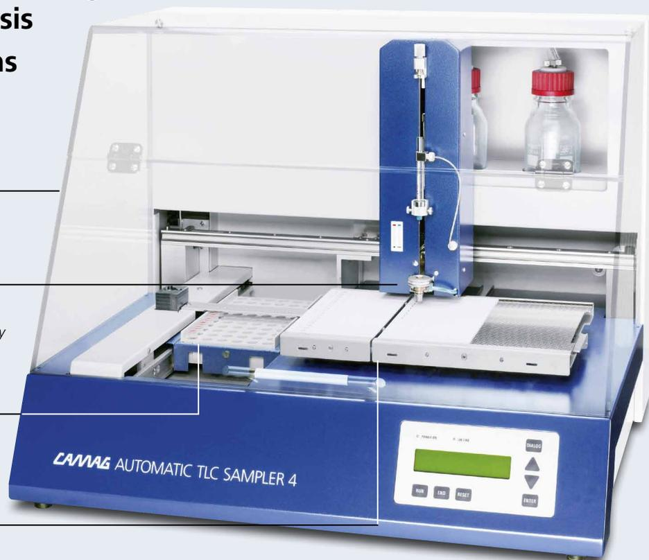
Automatic sample application is a key factor for high precision and productivity in routine analysis. With the ATS 4 the samples are either applied as spots through contact transfer (0.1–5  $\mu\text{L}$ ) or as bands using the spray-on technique (between 0.5 and > 50  $\mu\text{L}$ ). Large sample volumes can also be sprayed-on in the form of rectangles which are focused to narrow bands prior to chromatography.
