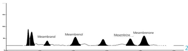
HPTLC densitogram of a sample (track 2) containing the four alkaloids
