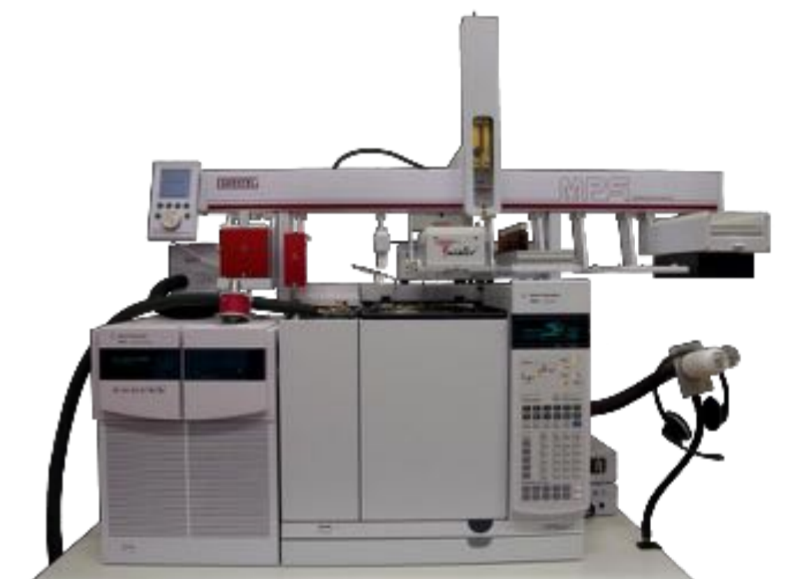
Figure 1: gas chromatograph with tandem mass spectrometer and olfactory detection port (GC-MS/MS-O)
