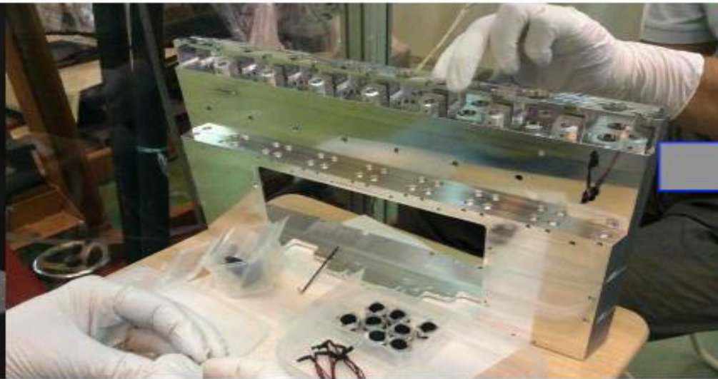
Enclosure: gluing CCDs and LEDs, integrating fiber mounts.
