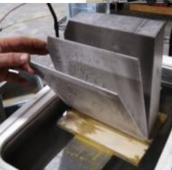
Wire Saw Cutting
