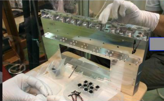
Enclosure: gluing CCDs and LEDs, integrating fiber mounts.
