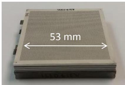
After potting, before readout PCB is attached
