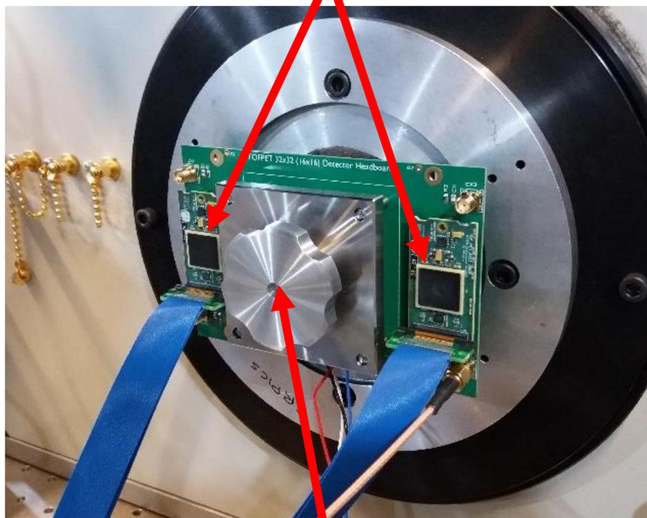
32 x 32 PMT with mechanically compressed ACF
