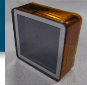
Hamamatsu 1" 16-ch MCP-PMT
