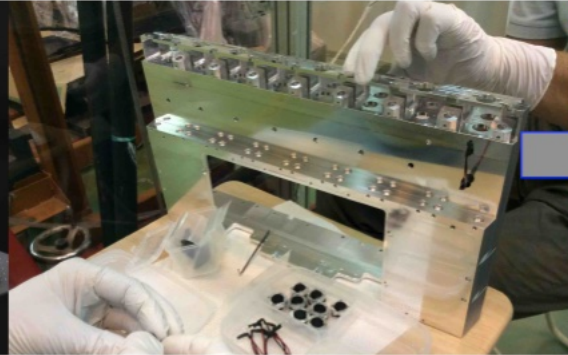
Enclosure: gluing CCDs and LEDs, integrating fiber mounts.
